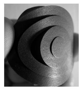
The deformation of the special material is less than 2% under long-term compression. Even after several years of use under e.g. a heavy loudspeaker its resonance damping properties will remain intact. The material is stable from  $\div 58 - 158^{\circ}F(\div 50 - 70^{\circ}C)$  and is furthermore chemically resistant to all commonly used household cleaning solvents.
