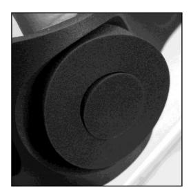
The deformation of the special material is less than 2% under long-term compression. Even after several years of use under e.g. a heavy loudspeaker its resonance damping properties will remain intact. The material is stable from  $\pm 58 - 158^\circ F (\pm 50 - 70^\circ C)$  and is furthermore chemically resistant to all commonly used household cleaning solvents.
